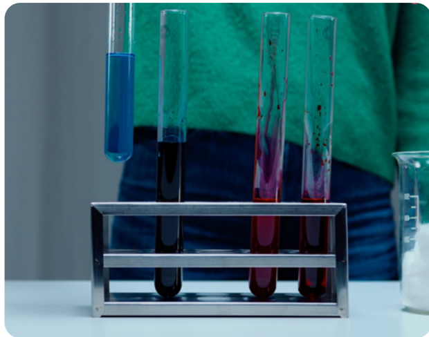
Fig. 9. Results of the Methylene Blue and Eosin Experiment Showing Soil Cation Retention
